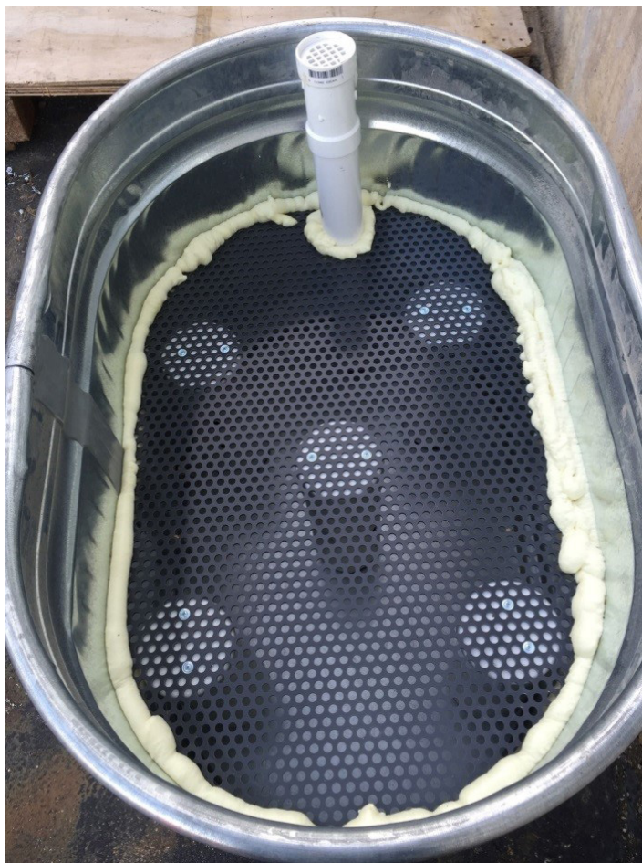
Figure 6. Perforated sheet with spray foam installed
