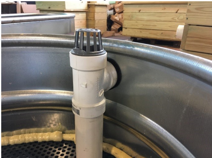
Figure 5a. Overflow riser installed with atrium grate
