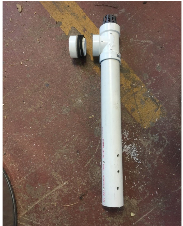
Figure 4. Overflow riser and through planter connection
