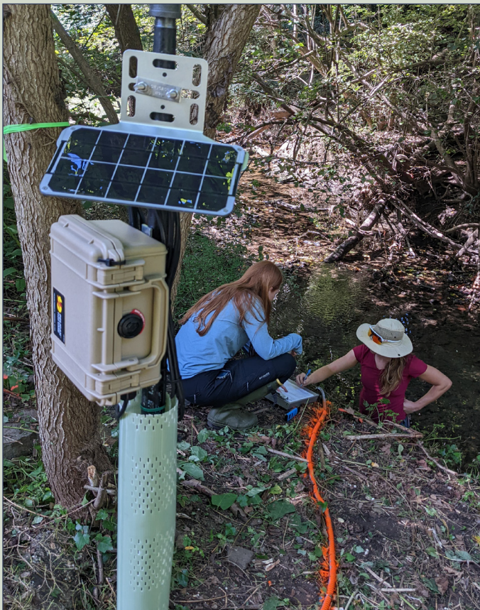
Stroud staff records the details of logger installation along Vine Creek.
