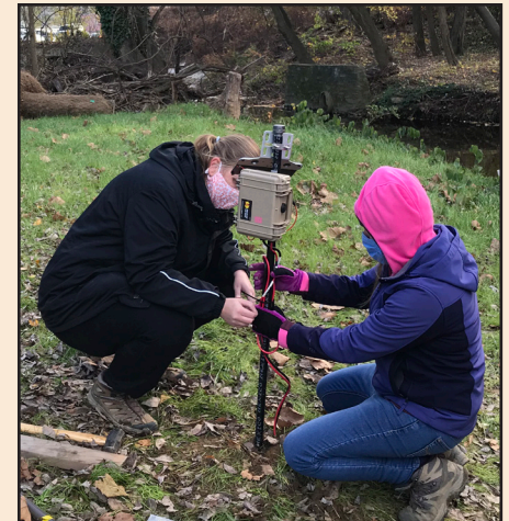
Conservancy Watershed Specialist Jamie Anderson and Pennsylvania Resources Council Eastern Program Director Diana Andrejczak install a stream monitoring station.
