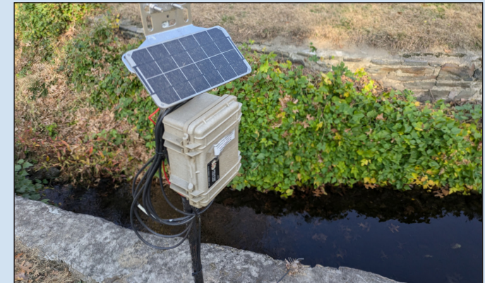
A logger installed at Elm Grove Park receives data from Indian Creek every fifteen minutes. View the data at monitormywatershed.org/sites/EBIC_shor/
